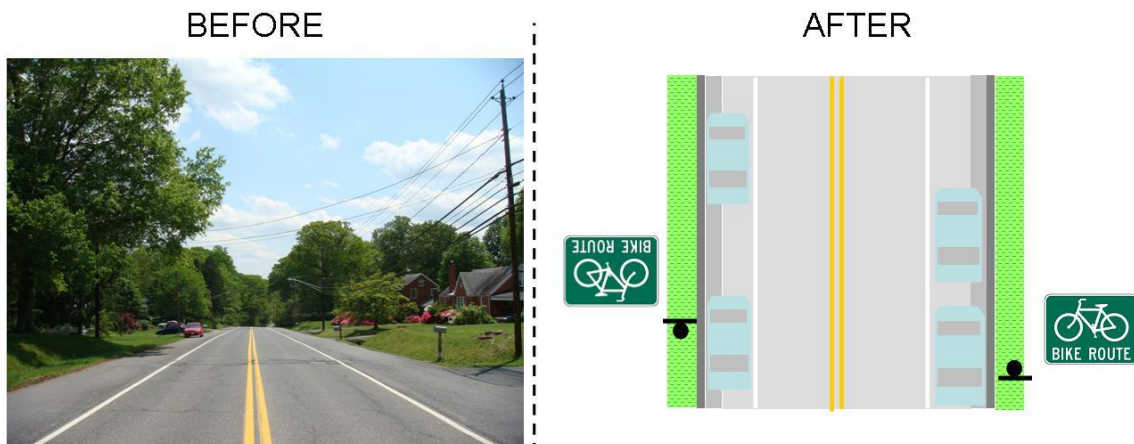
Figure 15: Before and After Signage/Striping Improvements for Brooklyn Bridge Rd.
