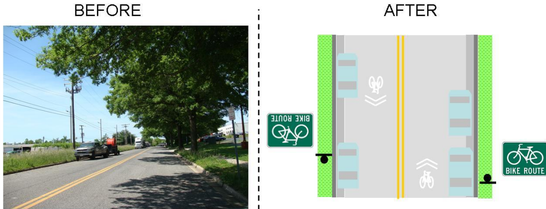
Figure 22: Before and After Signage/Striping Improvements for Staggers Lane
