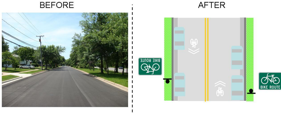
Figure 18: Before and After Signage/Striping Improvements for Laurelton Dr.
