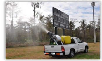
Barrier Treatment Application Equipment for Special Events and Larviciding Efforts
