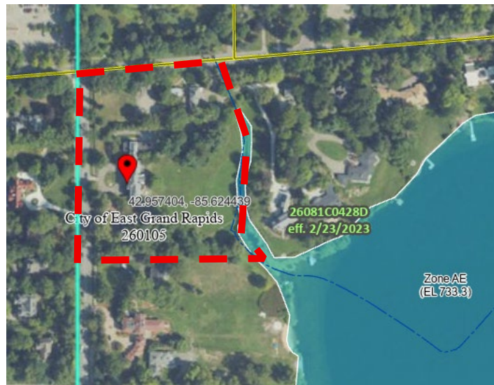
Exhibit 2 – FEMA Floodplain map for the area around Fisk Lake. 250 Plymouth boundary is shown in red above.
